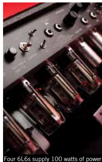
Four 6L6s supply 100 watts of power
