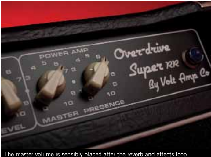
The master volume is sensibly placed after the reverb and effects loop
